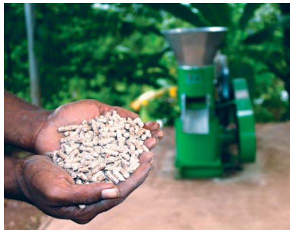
Pellet fuel from LitFuel, with the pelletizing machine seen in the background
